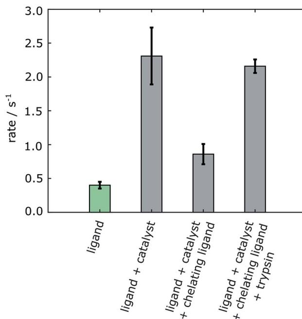
Fig. 4  $R_2$  relaxation rates of 4-amidinopyridine. The green bar is from a non-hyperpolarized experiment in the absence of polarization transfer catalyst. The gray bars are from 4-amidinopyridine hyperpolarized by SABRE. Errors are shown as standard deviations from three separate measurements taken from different samples (Table S1†).
