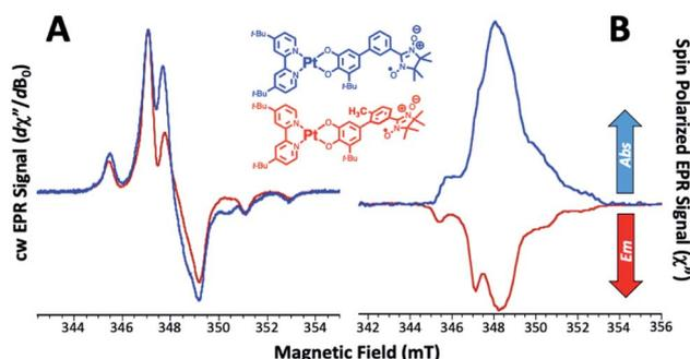
Fig. 4 X-band cw-EPR (A); 20 K; 2-MTHF, and TREPR (B); 20 K; 2-MTHF spectra for **mPh-Pt** (blue lines) and **6-Me-mPh-Pt** (red lines). (A) Field modulation detected cw-EPR spectra of the ground states without light excitation. (B) Light-induced, spin-polarized TREPR spectra, extracted from time/field datasets 4  $\mu\text{s}$  after the laser flash. Light excitation at 532 nm, concentrations  $\sim 0.5$  mM. Abs = absorption, Em = emission.
