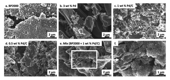
Fig. 3 SEM micrographs showing morphology of carbon supports. (a) BP2000 has uniform morphology with particle sizes in the nm range. (b-d) Pd/C have small particles as well as large agglomerates and micron size platelets. (e-f) The mix of {BP2000 + 1 wt% Pd/C} shows large agglomerates and platelets (likely Pd/C) that appear to be coated with small spherical particles (likely BP2000, see additional image in Fig. S9, ESI†).
