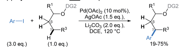
Scheme 7 Pd-catalysed directed \beta -C(sp 3 )-H arylations of alcohols using an O-N tethered directing group. 57
