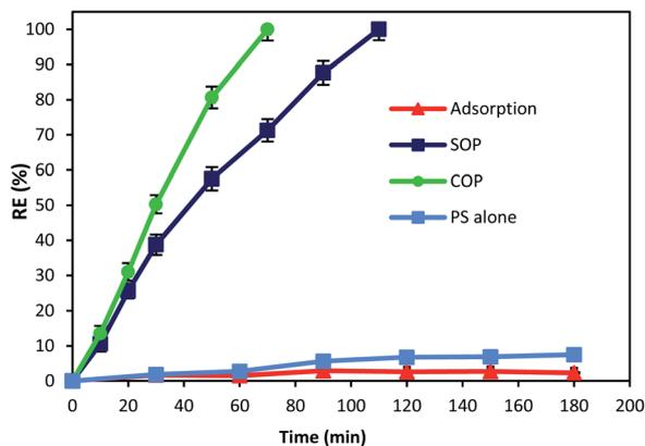
Fig. 6 Contribution of adsorption, SOP, COP and PS alone on cyanide removal (cyanide concentration:  $100 \text{ mg L}^{-1}$ , MgO concentration:  $500 \text{ mg L}^{-1}$ , ozone concentration:  $200 \text{ mg h}^{-1}$ , PS concentration:  $200 \text{ mg L}^{-1}$ , pH = 11, reaction time: 180 min).
