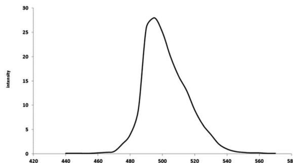
Fig. 10 Photoluminescence of the synthesized MgO.
