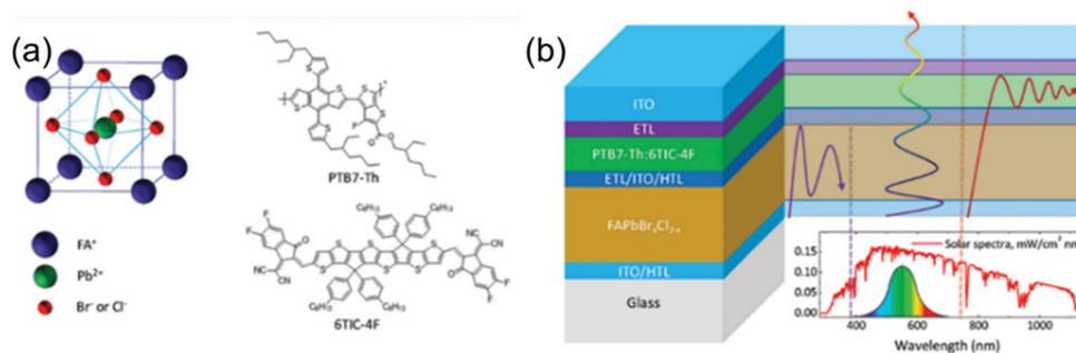
Fig. 17 (a) Scheme of FAPbBr<sub>x</sub>Cl<sub>3-x</sub> perovskite crystal lattice, Chemical structures of PTB7-Th and 6TIC-4F. (b) Device architectures of selective absorbing tandem ST-PVs.<sup>85</sup>
