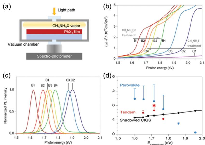
Fig. 16 (a) Scheme of *in situ* bandgap tuning apparatus. (b) Tauc plots of sample series B and C, showing a blueshift progression with  $\text{CH}_3\text{NH}_2\text{Br}$  vapor treatment and a redshift progression with  $\text{CH}_3\text{NH}_2\text{I}$  vapor treatment, respectively. (c) PL spectra of series B and C. (d) Efficiency plotted against the bandgap of perovskite.<sup>69</sup>
