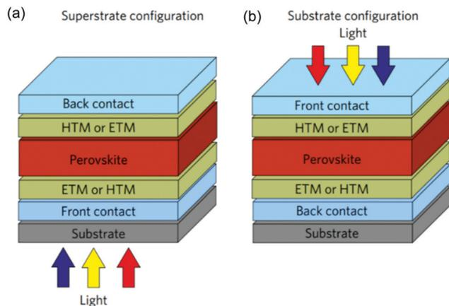
Fig. 14 Scheme of a perovskite solar cell in the (a) conventional superstrate configuration and (b) the substrate configuration.<sup>67</sup>
