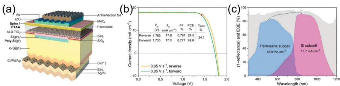
Fig. 7 (a) Scheme of the interlayer-free monolithic perovskite–c-Si tandem solar cell. (b)  $J-V$  curve of the tandem device with both reverse and forward scanning at  $0.05\text{ V s}^{-1}$  based on heterojunction poly-Si subcell. (c) Absorbance (1–reflectance) of the tandem device (gray), EQE of the perovskite top cell (blue), and the c-Si bottom subcell (pink).<sup>29</sup>
