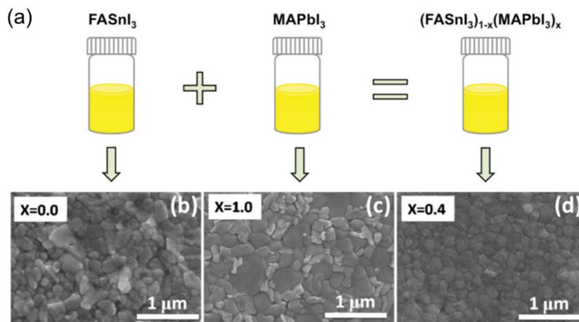
Fig. 12 (a) Scheme of the formation of (FASnI<sub>3</sub>)<sub>1-x</sub>(MAPbI<sub>3</sub>)<sub>x</sub> precursor. (b–d) SEM images of (FASnI<sub>3</sub>)<sub>1-x</sub>(MAPbI<sub>3</sub>)<sub>x</sub> perovskite films ( $x = 0.0, 1.0, \text{ and } 0.4$ ).<sup>58</sup>
