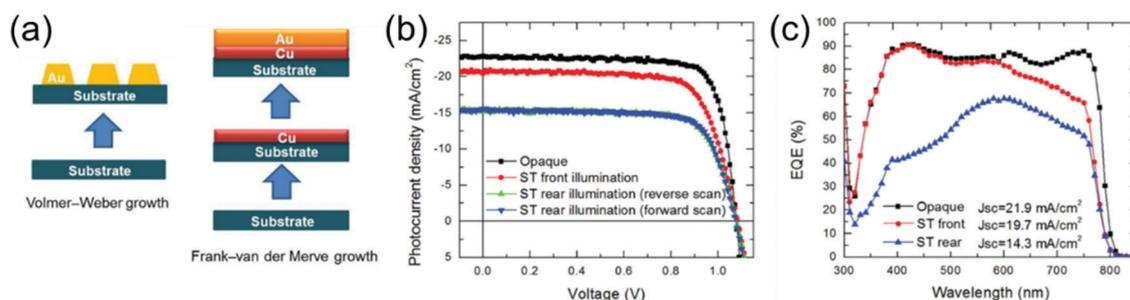
Fig. 3 (a) Scheme of Volmer-Weber growth and Frank-van der Merve growth. (b)  $J$ - $V$  curves of opaque and semitransparent PSCs. (c) EQE curves of opaque and ST-PSCs under front and rear illumination.<sup>16</sup>
