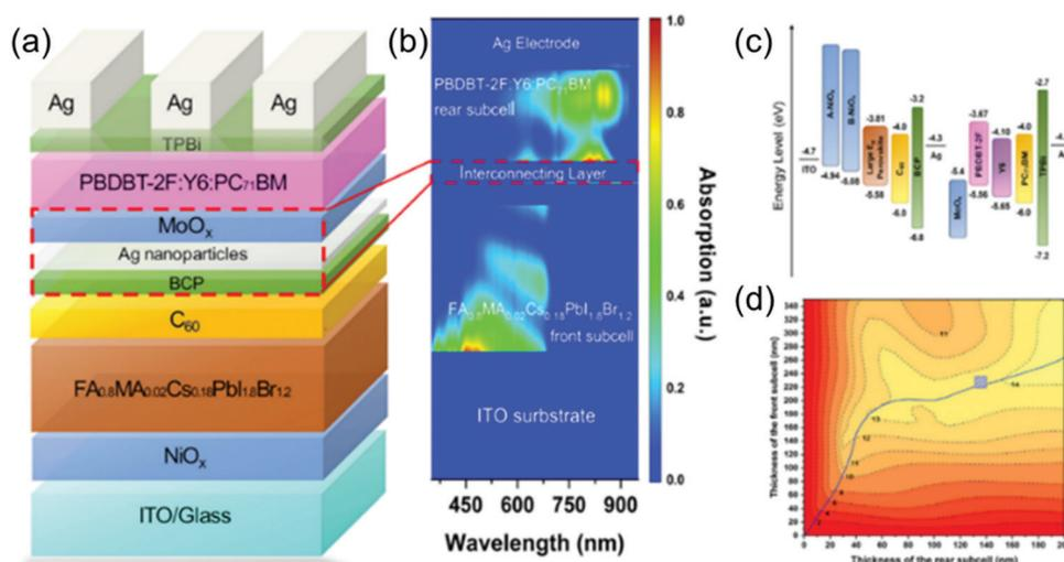
Fig. 18 (a) Perovskite–organic tandem structure with an ICL of MoO<sub>x</sub>/Ag nanoparticles/BCP. (b) The simulation of the photon absorption distribution in tandem. (c) Energy level distribution of the components in the tandem device. (d) Stimulated current density as a function of the thicknesses of the front and rear subcells.<sup>88</sup>
