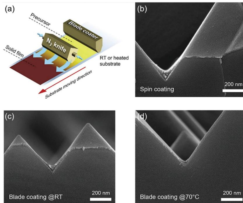
Fig. 9 (a) Scheme of  $N_2$ -assisted blade coating. (b–d) SEM images of PTAA on textured silicon bottom cells deposited by (b) spin coating, (c)  $N_2$ -assisted blade coating with the substrate at room temperature, and (d)  $N_2$ -assisted blade coating with the substrate at  $70^\circ\text{C}$ . The three visible layers are the silicon wafer, ITO front electrode of the silicon cell, and PTAA hole-transport layer.<sup>33</sup>
