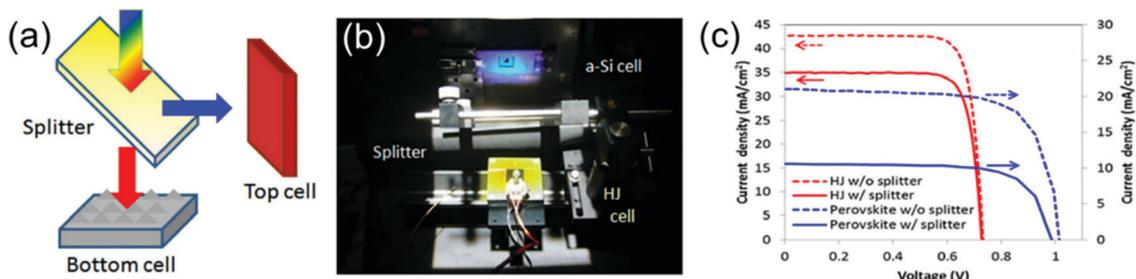
Fig. 5 (a) Scheme of the optical splitting system, (b) measurement setup of an optical splitting system, and (c)  $J$ – $V$  curves of SHJ and perovskite solar cells with and without a splitter.<sup>22</sup>
