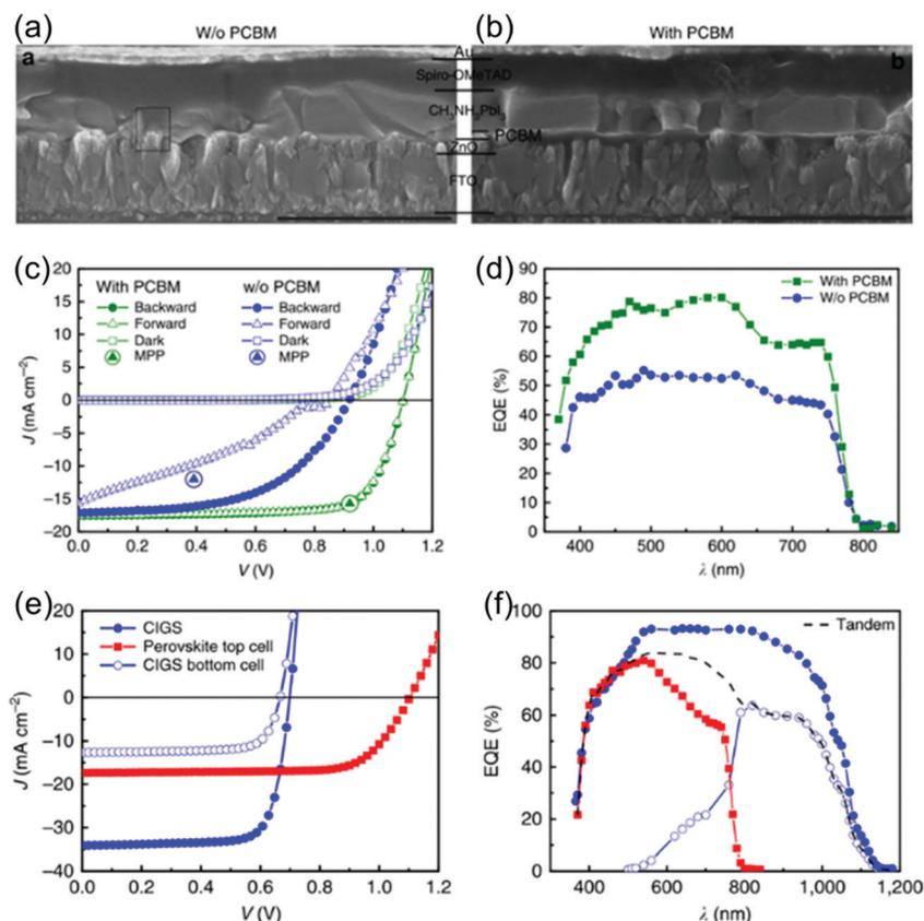
Fig. 15 The cross-sectional SEM images of devices without (a) and with (b) PCBM, respectively. The current density–voltage ( $J$ – $V$ ) curves (c) and EQE spectra (d) of the planar perovskite solar cells. The current density–voltage ( $J$ – $V$ ) curves (e) and EQE spectra (f) of the four-terminal perovskite–CIGS tandem device.<sup>68</sup>
