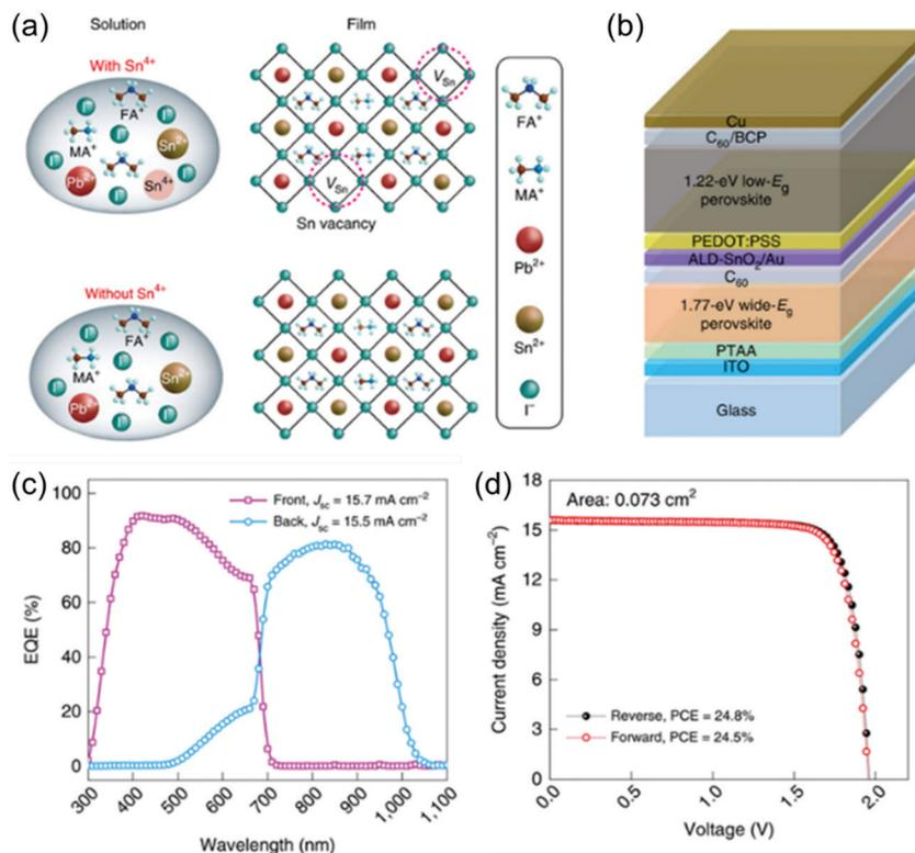
Fig. 13 (a) Scheme of the formation of Sn vacancies in mixed Sn–Pb perovskite due to the presence of Sn<sup>4+</sup> in the precursor solution and the suppression of Sn vacancy formation because of the absence of Sn<sup>4+</sup>. (b) The device architecture of the perovskite–perovskite tandem solar cell. (c) EQE curves of the front (15.7 mA cm<sup>-2</sup>) and back (15.5 mA cm<sup>-2</sup>) subcells. (d) *J*–*V* curves of the tandem solar cell (0.049 cm<sup>2</sup>).<sup>63</sup>
