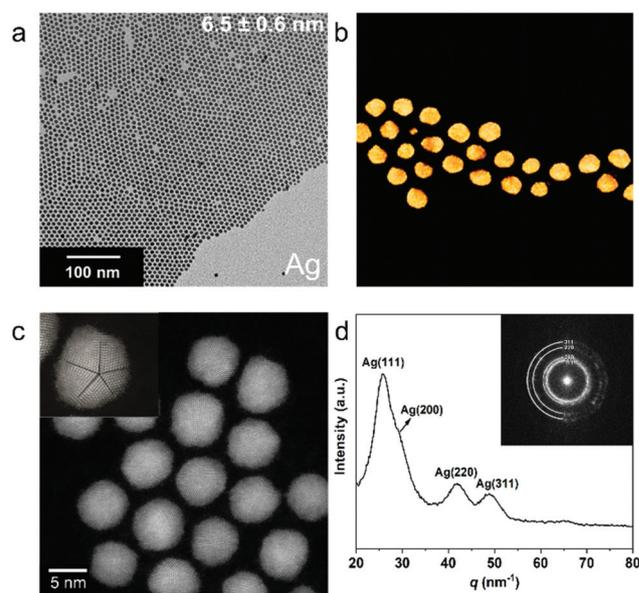
**Fig. 2** (a) TEM image of colloidal Ag NPs. (b) 3D visualization of the reconstructed volume of a number of Ag NPs. (c) High resolution HAADF-STEM image of Ag NPs, showing the polycrystallinity of the NPs and the presence of pentatwinned domains. A magnified image of a region with a pentatwinned domain is shown as inset. (d) Fourier transform (FT) pattern (inset) of Ag NPs and the radially integrated 1D Powder Electron Diffraction (PED) pattern.
