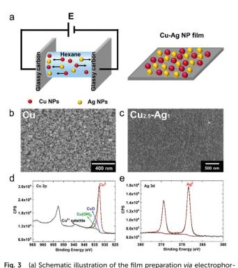
esis. The arrows indicate the moving direction of NPs under applied potential. (b and c) SEM images of the anode Cu (b) and Cu<sub>2.5</sub>-Ag<sub>1</sub> (c) NPs film prepared at 100 V for 60 min. (d and e) Cu 2p (d) and Ag 3d (e) XPS spectra of a Cu<sub>2.5</sub>-Aq<sub>1</sub> NPs film prepared by electrophoresis at 100 V for 60 min.
