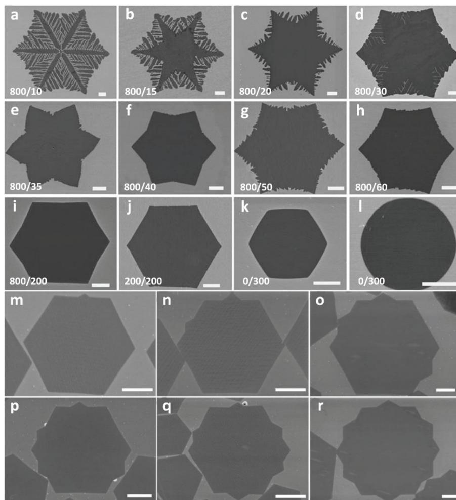
**Fig. 5** SEM images of GFs grown on a liquid Cu surface with different shapes formed by varying the Ar : H<sub>2</sub> ratio (a–l). Reprinted with permission from Springer Nature, NPG Asia Materials<sup>74</sup> (self-organized graphene crystal patterns, B. Wu *et al.*, 2013). Formation of tips in hexagonal graphene grains by incremental additions to the CH<sub>4</sub> flow (m–r). Reprinted with permission from ref. 75. Copyright 2014 Wiley-VCHd. All scale bars are 5 μm.
