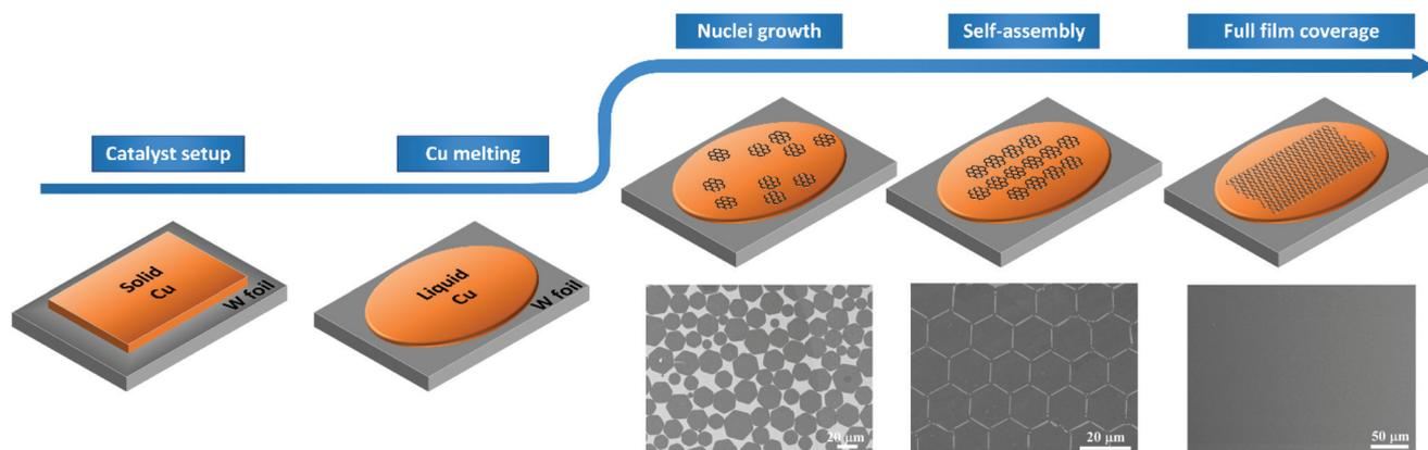
**Fig. 1** Schematic illustration of the CVD growth process of graphene on liquid Cu. SEM images are indicative of dispersed graphene hexagonal flakes, self-ordered graphene hexagonal flakes and continuous uniform graphene film, respectively (this figure has been adapted/reproduced from ref. 42 with permission from PNAS, copyright 2012).
