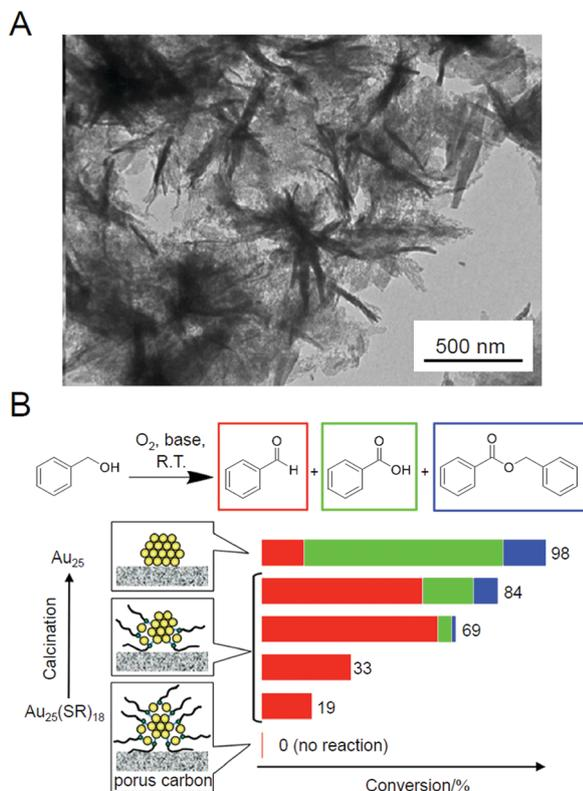
Fig. 5 (A) TEM image of HPCs. (B) Catalytic performance of  $\text{Au}_{25}(\text{SC12})_{18-x}/\text{HPCs}$  for aerobic oxidation of benzyl alcohol. Reproduced with permission from ref. 210. Copyright 2014 American Chemical Society.
