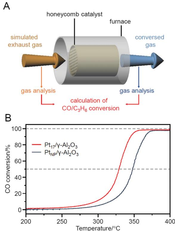
Fig. 22 (A) Schematic of the estimation of CO conversions over  $\text{Pt}_{17}/\gamma\text{-Al}_2\text{O}_3$  or  $\text{Pt}_{\text{NP}}/\gamma\text{-Al}_2\text{O}_3$  coated on a cordierite honeycomb substrate. (B) CO conversions over  $\text{Pt}_{17}/\gamma\text{-Al}_2\text{O}_3$  or  $\text{Pt}_{\text{NP}}/\gamma\text{-Al}_2\text{O}_3$ . Reproduced from ref. 235. Copyright 2020 Royal Society of Chemistry.
