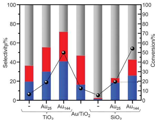
**Fig. 11** Catalytic activity of loaded Au<sub>25</sub> and Au<sub>144</sub> NCs (pre-treated at 150 °C) in cyclohexane oxidation. Cyclohexane conversion normalized to the Au loading (except for the blank measurements) (right axis); product distribution (left axis): red, blue, and gray represent cyclohexanol, cyclohexanone, and by-products, respectively. Reproduced with permission from ref. 218. Copyright 2019 Elsevier.
