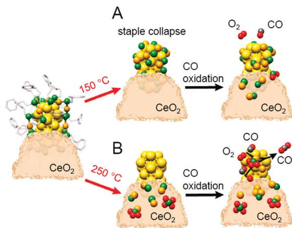
Fig. 19 Evolution of  $\text{Au}_{38}(\text{PET})_{24}/\text{CeO}_2$  catalyst structure estimated from EXAFS analyses: catalysts after pre-treatment at (A) 150 °C and (B) 250 °C and subsequent CO oxidation. Reproduced with permission from ref. 233. Copyright 2020 American Chemical Society.
