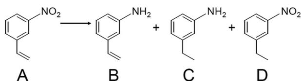
Scheme 10 Hydrogenation of 3-nitrostyrene using metal catalysts. The reaction was conducted under  $\text{H}_2$  atmosphere in toluene. A = 3-nitrostyrene, B = 3-vinylniline, C = 3-ethylaniline, D = 3-ethylnitrobenzene.
