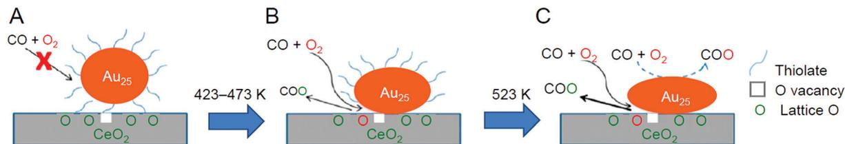
Fig. 18 CO oxidation mechanism on (A) intact, (B) partially dethiolated, and (C) fully dethiolated  $\text{Au}_{25}(\text{PET})_{18}/\text{CeO}_2$  catalysts. Reproduced with permission from ref. 231. Copyright 2014 American Chemical Society.
