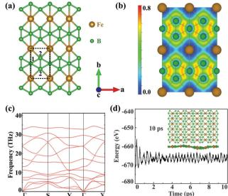
Fig. 1 (a) Geometric structures, (b) ELF, (c) phonon spectrum and (d) AIMD simulations for the  $\alpha$ -FeB $_3$  monolayer. The brown and green spheres represent Fe and B atoms, respectively. The top and side views of  $\alpha$ -FeB<sub>3</sub> at the end of the AIMD simulation are shown in (d).
