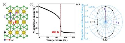
Fig. 2 (a) Spin-dependent charge density of the  $\alpha$ -FeB<sub>3</sub> monolayer, (b) average magnetic moment as a function of temperature and (c) MAE in the x-yplane with respect to the out-of-plane direction. The isovalue of the spin charge density is set to be 0.01 e  ${\rm \AA}^{-3}$ .
