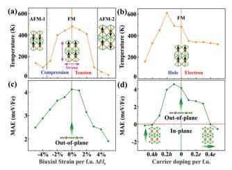
Fig. 3 Transition temperature and magnetic anisotropy energy (MAE) of the FeB<sub>3</sub> monolayer as a function of (a and c) external strains and (b and d) charge-carrier doping, respectively.
