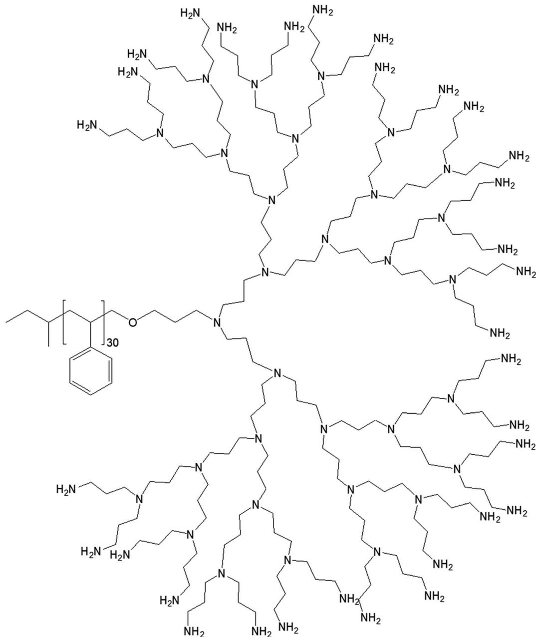
Fig. 10 Chemical structure of polystyrene conjugated to the highest generation poly(propylene imine) dendrimer PS-dendr-(NH<sub>2</sub>)<sub>32</sub>.
