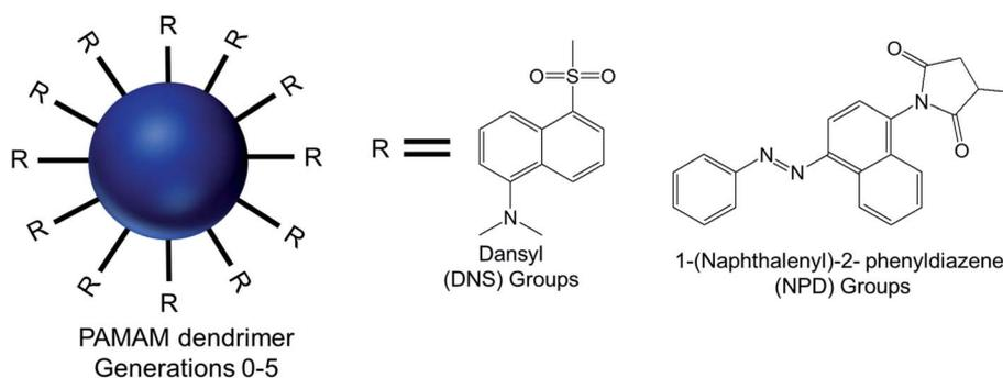
Fig. 16 Chemical structure of modified generation 0 to 5 PAMAM dendrimers conjugated to hydrophobic aromatic dansyl (DNS) or 1-(naphthalenyl)-2-phenyldiazene (NPD) groups, *via* sulfonylation and a Michael addition reaction respectively.
