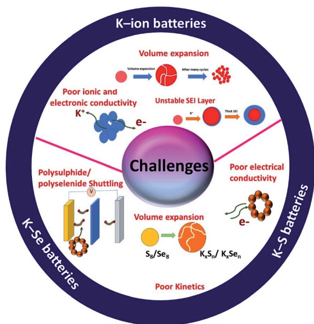
Fig. 3 Schematic of the challenges of potassium batteries.
