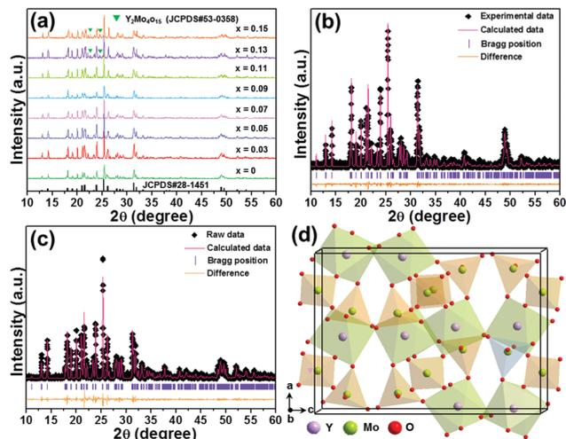
Fig. 1 (a) XRD patterns of the  $\text{Y}_2\text{Mo}_3\text{O}_{12}:\text{Er}^{3+}/2x\text{Yb}^{3+}$  microparticles. Rietveld XRD refinement patterns of the (b)  $\text{Y}_2\text{Mo}_3\text{O}_{12}:\text{Er}^{3+}$  and (c)  $\text{Y}_2\text{Mo}_3\text{O}_{12}:\text{Er}^{3+}/0.22\text{Yb}^{3+}$  microparticles. (d) Crystal structure of the  $\text{Y}_2\text{Mo}_3\text{O}_{12}$  unit cell.
