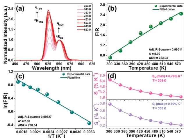
Fig. 4 (a) Normalized green UC emission spectra of the  $\text{Y}_2\text{Mo}_3\text{O}_{12}:\text{Er}^{3+}/0.22\text{Yb}^{3+}$  microparticles in the temperature range of 303–583 K. (b) Temperature-dependent FIR value. (c) Plot of  $\ln(\text{FIR})$  versus  $1/T$  of the  $\text{Y}_2\text{Mo}_3\text{O}_{12}:\text{Er}^{3+}/0.22\text{Yb}^{3+}$  microparticles. (d) Dependence of the  $S_a$  and  $S_r$  values on the temperature.
