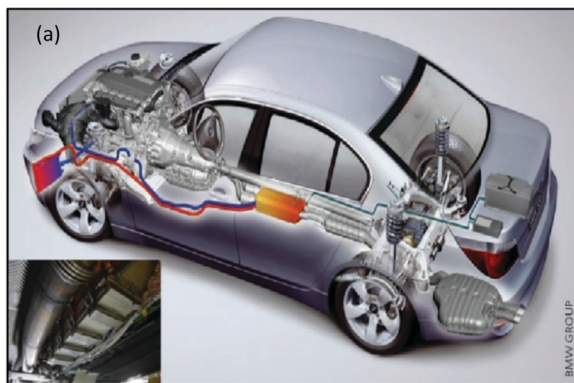
Fig. 18 Integration of thermoelectrics into vehicles for improved fuel efficiency. The image is a BMW 530i concept car with a thermoelectric generator (yellow; and inset) and radiator (red/blue). Reprinted by permission from (Springer Nature), (Nat. Mater.) ref. 182 (An inconvenient truth about thermoelectrics, C. B. Vining, 8 (2009) 83–85), Copyright 2009.
