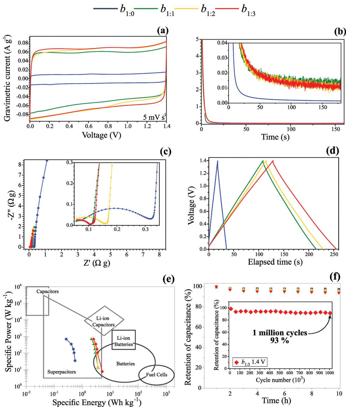
**Fig. 5** Electrochemical data and performance of the symmetric coin cell as a function of the MWCNT:AC mass ratio: (a) cyclic voltammograms at 5 mV s<sup>-1</sup>, (b) transient currents during the SSC experiments at 1.4 V, (c) EIS at 1.4 V, (d) GCD at 0.15 A g<sup>-1</sup>, (e) the Ragone plot, and (f) capacitance retention after 1 million cycles. Electrolyte: 1.0 mol dm<sup>-3</sup> Li<sub>2</sub>SO<sub>4</sub>.
