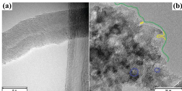
Fig. 2 TEM images obtained from the (a) MWCNT and (b) AC carbon materials. We highlighted an example of the AC macropore in green, mesopores in yellow and micropores in blue.
