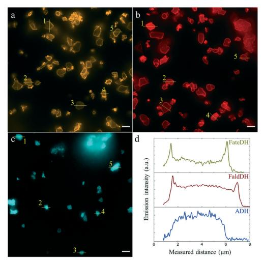
Fig. 2 The individual enzyme distribution along the MCF particle in separate sets of individual enzyme immobilizations. The scale bar is 5 µm. (a) FateDH-Cy3, (b) FaldDH-Cy5, (c) ADH-AF488. (d) Emission intensity profiles of particles labelled #1 in a (yellow), b (red), c (blue). All the profiles are shown in Fig. S3.†
