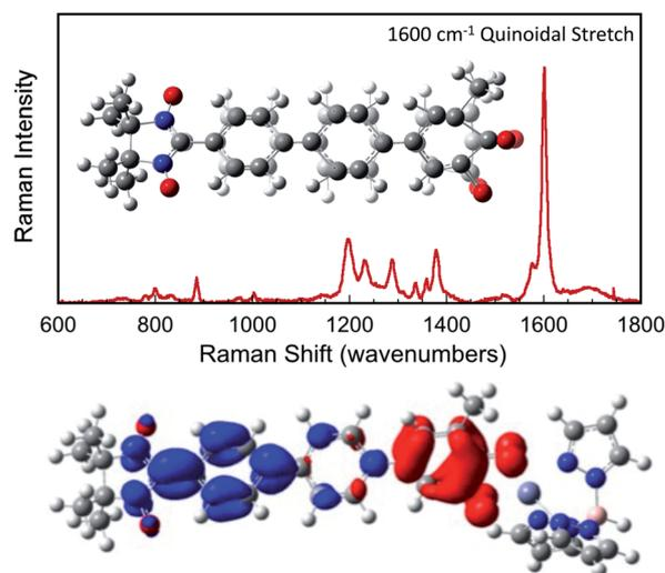
Fig. 8 Top: Resonance Raman spectrum collected on resonance with the SQ  $\rightarrow$  Ph-NN ILCT band showing large resonance enhancement of the  $1600 \text{ cm}^{-1}$  quinoidal stretch (inset). Bottom: Computed electron density difference map (EDDM) that highlights the nature of the SQ  $\rightarrow$  Ph-NN ILCT. Electron density loss in the transition is shown in red, while the electron density gain is shown in blue.
