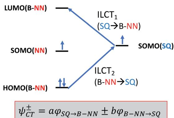
Fig. 3 Simple 4-orbital diagram showing NN-Bridge(HOMO)  $\rightarrow$  SQ(SOMO) and SQ(SOMO)  $\rightarrow$  NN-Bridge(LUMO) one-electron promotions that figure prominently in charge transfer configurations that contribute to magnetic exchange in SQ-Bridge-NN biradicals.
