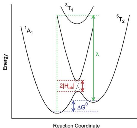
Fig. 3 Generalized potential energy surface diagram for a low-spin  $d^6$  complex of O symmetry whose kinetics can be described by eqn (1). Electronic coupling between the  $S = 0$  and  $S = 2$  states is facilitated *via* mixing with a (thermally inaccessible) excited  $S = 1$  state, resulting in an avoided crossing on the lower potential surface. The reorganization energy indicated corresponds to that associated with the  $^5\text{T}_2 \rightarrow ^1\text{A}_1$  conversion.
