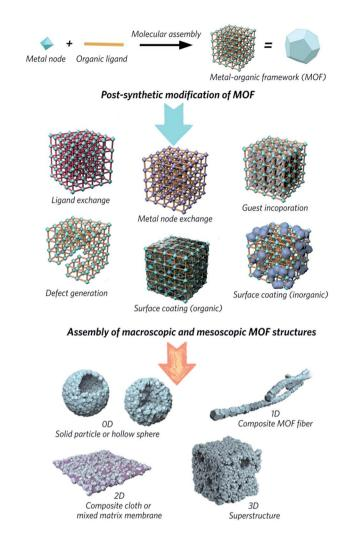
Fig. 1 Schematic overview of post-synthetic modifications and meso/ macroscopic morphological assemblies of MOFs.
