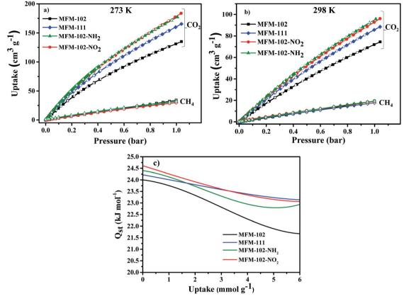
Fig. 2 Adsorption isotherms for desolvated MFM-102, MFM-111, MFM-102-NO<sub>2</sub> and MFM-102-NH<sub>2</sub> (a) 273 K, (b) 298 K. Solid and open symbols represent adsorption and desorption, respectively. (c) Heat of adsorption as a function of CO2 uptake derived by the virial method.
