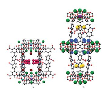
Fig. 4 The positions of the  $CO_2$  in the framework cage A (a) and B (b) of MFM-102-NO<sub>2</sub>.  $CO_2$  molecules are at site I (yellow), site II (green), site III (brown), site IV (ruby), site V (blue) and site VI (purple).
