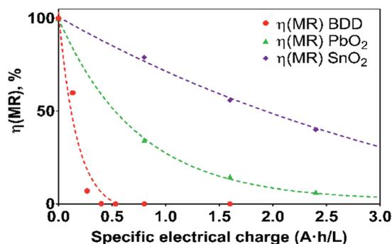
Fig. 7 Current efficiency ( $\eta$ ) values for the electrooxidation of MR as a function of the specific electrical charge ( $\text{A h L}^{-1}$ ) for solutions containing  $20 \text{ mg L}^{-1}$  MR in  $0.5 \text{ M H}_2\text{SO}_4$  at  $30 \text{ mA cm}^{-2}$  and  $298 \text{ K}$ : ● Si/BDD, ◆ Ti/Sb-doped  $\text{SnO}_2$ , ▲ Pb/PbO<sub>2</sub>.
