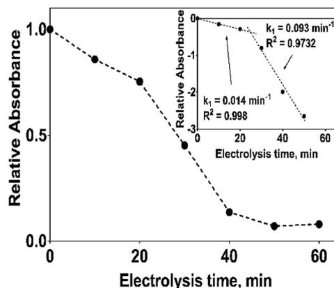
Fig. 9 Plot of the relative absorbance at 285 nm of 2,4-DNa as a function of the electrolysis time for the electrolysis of a solution containing  $100 \text{ mg L}^{-1}$  2,4-DNa in  $0.5 \text{ M Na}_2\text{SO}_4$  at  $30 \text{ mA cm}^{-2}$  and  $298 \text{ K}$  on Si/BDD anode. Inset shows the corresponding pseudo-first order graphic.
