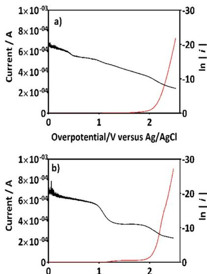
Fig. 11 The variation of current as a function of the overpotential ( $\eta$ ) for BDD in (a) 0.5 M Na<sub>2</sub>SO<sub>4</sub> solution and (b) 0.5 M Na<sub>2</sub>SO<sub>4</sub> + 100 ppm 2,4-DNa (pH 3) solution at 10 mV s<sup>-1</sup> and 298 K. Tafel curves are included for each one of the cases plotting  $\ln(i)$  against  $\eta$  (black curves).
