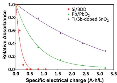
Fig. 6 Plots of the relative absorbance of MR against specific electrical charge ( $\text{A h L}^{-1}$ ) for solutions containing  $20 \text{ mg L}^{-1}$  MR in  $0.5 \text{ M H}_2\text{SO}_4$  at  $30 \text{ mA cm}^{-2}$  and  $298 \text{ K}$ : ● Si/BDD, ◆ Ti/Sb-doped  $\text{SnO}_2$ , ▲ Pb/PbO<sub>2</sub>.
