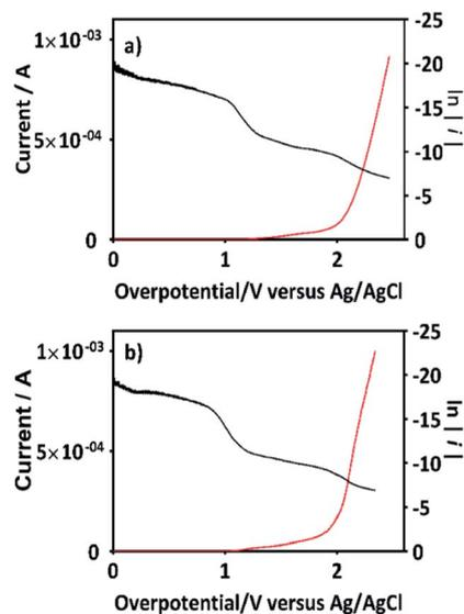
Fig. 13 The variation of current as a function of the overpotential ( $\eta$ ) for BDD in (a) 0.5 M  $\text{NaClO}_4$  solution and (b) 0.5 M  $\text{NaClO}_4$  + 100 ppm 2,4-DNa (pH 3) solution at 10  $\text{mV s}^{-1}$  and 298 K. The Tafel analysis is included for each one case in the corresponding figure (plotting  $\ln(i)$  against  $\eta$ ).
