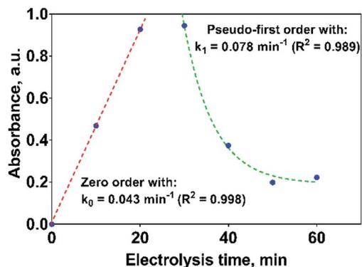
Fig. 10 Kinetic parameters for the formation and consumption of 2,4-DP as first reaction intermediate on the Si/BDD anode in 0.5 M Na<sub>2</sub>SO<sub>4</sub> + 100 ppm 2,4-DNa solution at 30 mA cm<sup>-2</sup> and 298 K.
