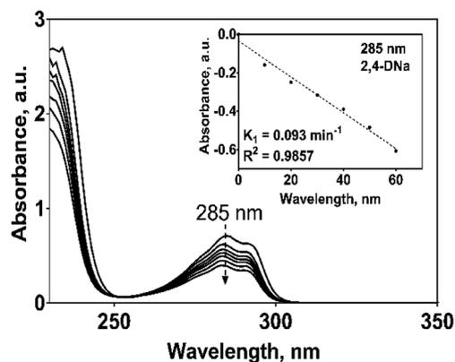
Fig. 12 UV spectra, as a function of the electrolysis time, for 100  $\text{mg L}^{-1}$  2,4-DNa solutions in 0.5 M  $\text{NaClO}_4$  electrolyzed on a Si/BDD anode at 30  $\text{mA cm}^{-2}$  and 298 K. Inset shows the pseudo-first order graphic of the UV band decrease at 285 nm.
