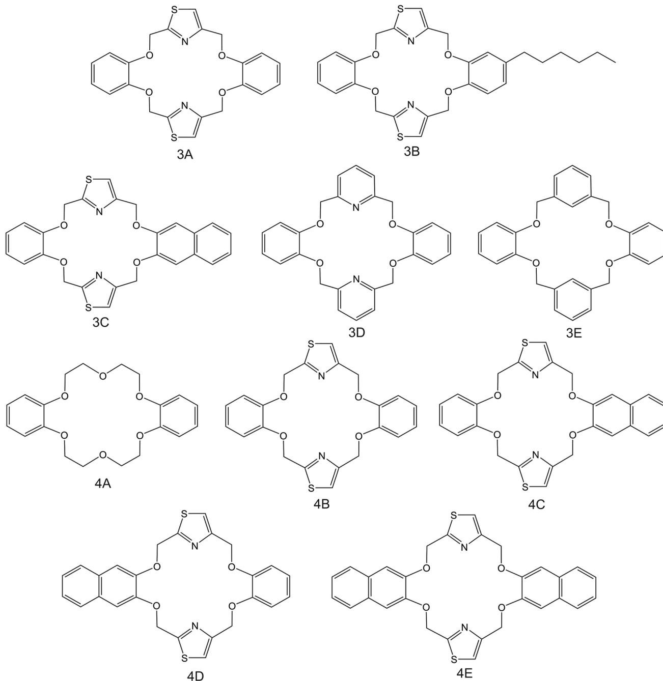
Fig. 4 DB18C6 derivatives, reported in the works by Kim *et al.* (3A–3E,<sup>83</sup> 4A–4E<sup>85</sup>), as  $\text{NH}_4^+$  ionophores.
