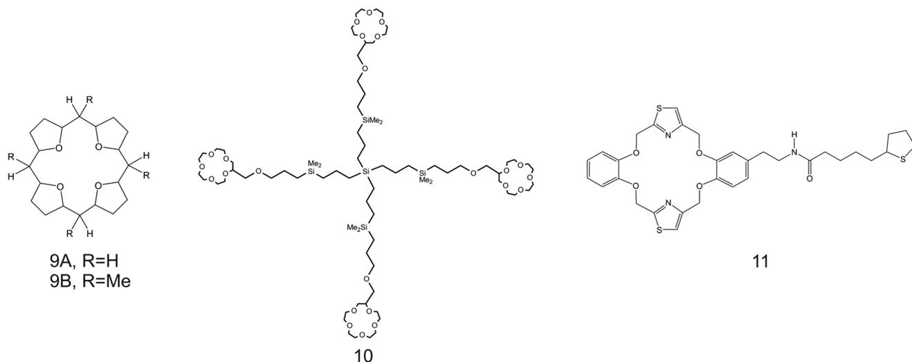
Fig. 8 THF-containing 16-crown-4 derivative (9A and 9B), 15-crown-5 substituted carbosilane dendrimer (10), and DB18C6 (11) reported in the works of Jin *et al.*,<sup>90</sup> Chandra *et al.*,<sup>91</sup> and Jin *et al.*,<sup>92</sup> respectively, as  $\text{NH}_4^+$  ionophores.
