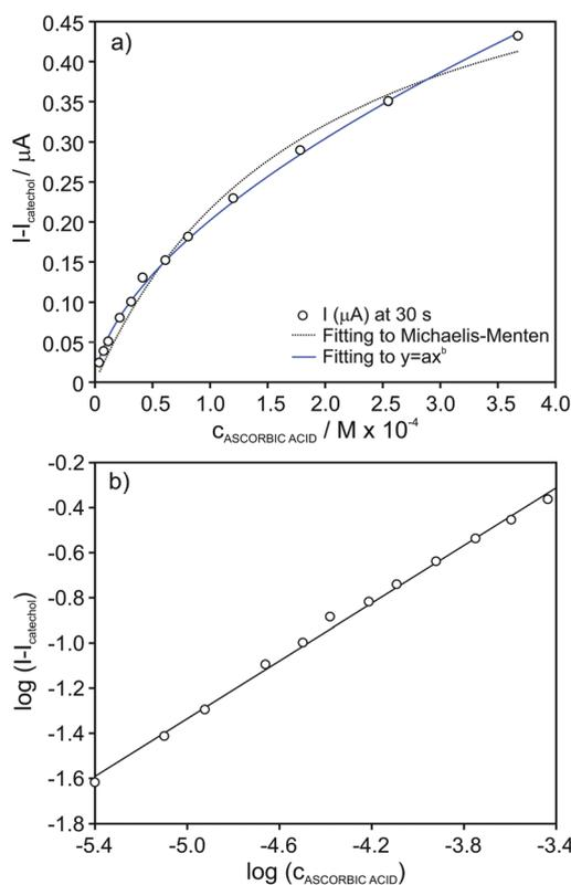
Fig. 6 (a) Plot of the absolute current change for increasing concentration of ascorbic acid in the presence of  $4 \times 10^{-5}$  M catechol concentration. (b) Calibration graph after data linearization.
