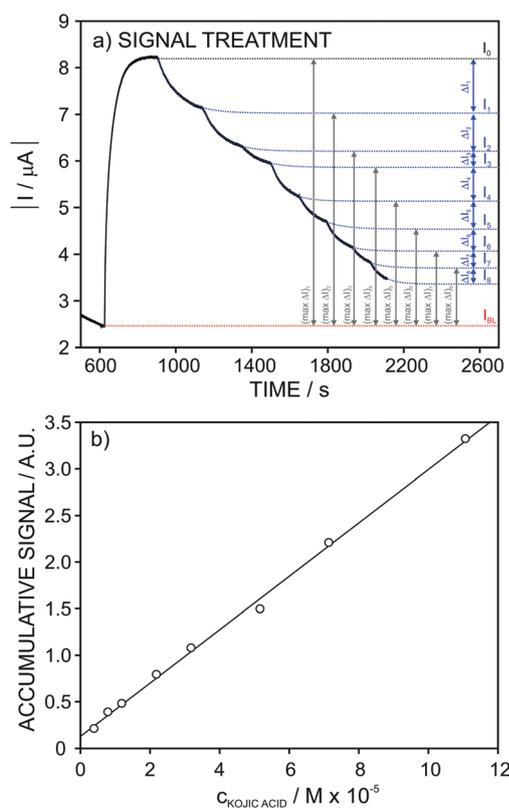
**Fig. 8** (a) Recorded current response for increasing kojic acid concentration (black) and the corresponding extrapolated fitted curves (dashed blue line). (b) Calibration graph observed after linearization.
