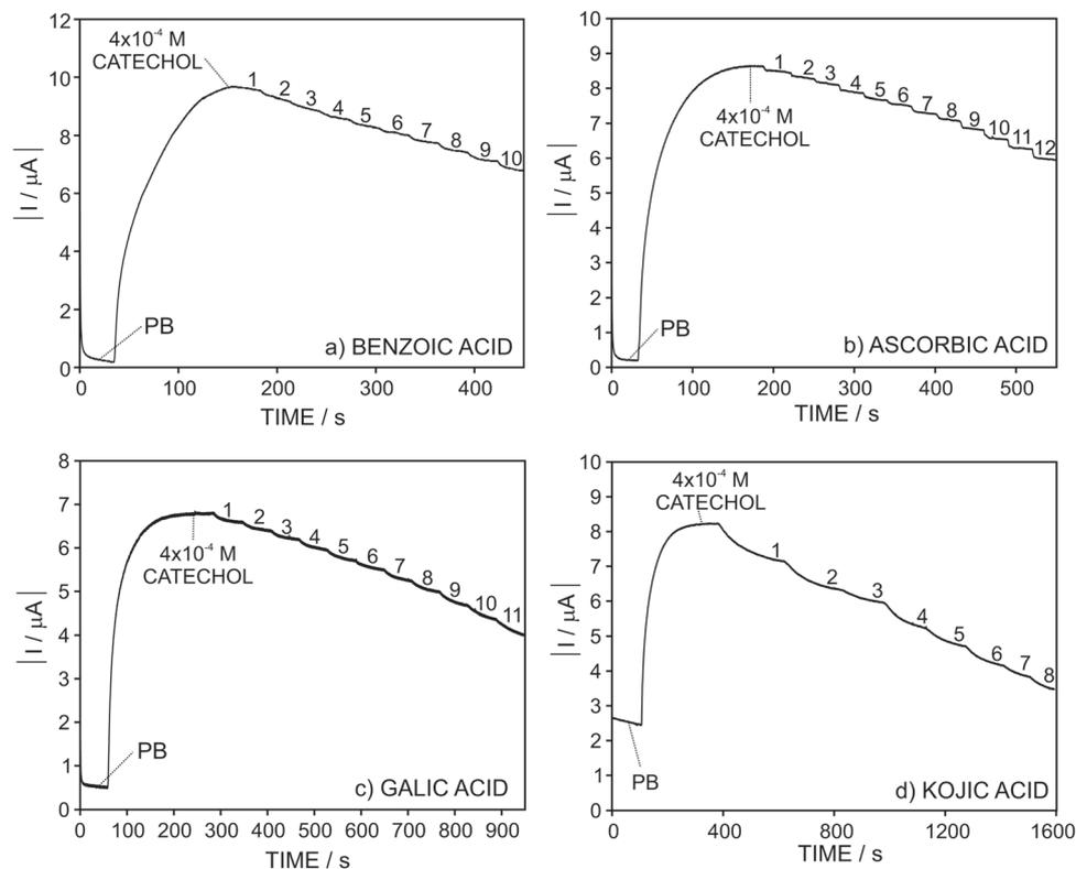
Fig. 4 Dynamic response of the sensors at a fixed concentration of catechol ( $4 \times 10^{-4} \text{ M}$ ) and gradually increasing the inhibitor concentration in the solution: (a) benzoic acid, (b) ascorbic acid, (c) gallic acid, and (d) kojic acid.
