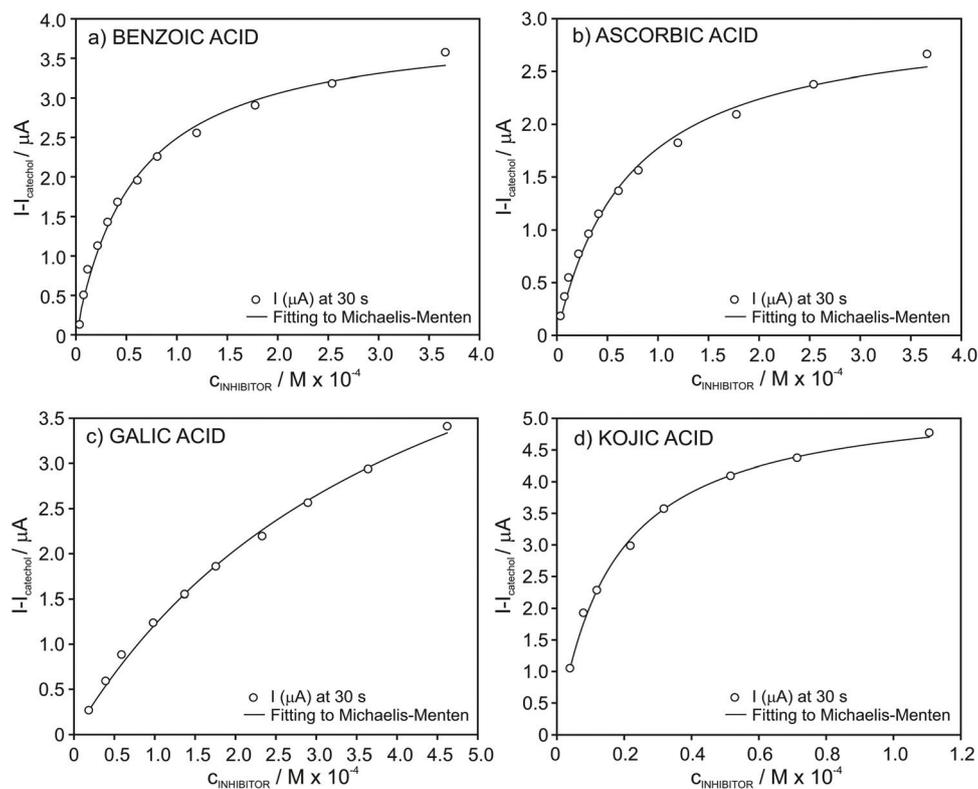
Fig. 5 Plot of the absolute current change for increasing concentrations of the inhibitors in the presence of  $4 \times 10^{-4} \text{ M}$  catechol concentration in PB: (a) benzoic acid, (b) ascorbic acid, (c) gallic acid, and (d) kojic acid.
