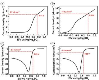
Fig. 2 Linear scan voltammograms of the n-GaAs electrode and Pt electrode at a scan rate of 100 mV s $^{-1}$ : (a) and (c) in the dark; (b) and (d) under illumination. The aqueous solution contains 40 mM KMnO₄ and 1.84 M H<sub>2</sub>SO<sub>4</sub>. The working temperature is kept at 25 °C and the illumination power is 460 mW.
