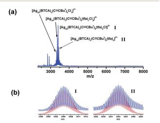
Fig. 2 (a) Mass spectrum of cluster 1. (b) The measured (blue trace) and simulated (red trace) isotopic patterns of [Ag<sub>34</sub>(BTCA)<sub>3</sub>(- $C \equiv CBu^t)_0(tfa)_2Cll^{2+}$  (I) and  $[Aq_{34}(BTCA)_3(C \equiv CBu^t)_0(tfa)_3]^{2+}$  (II).
