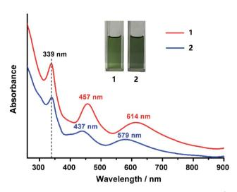
Fig. 4 The optical absorption spectra of  $[Ag_{34}(BTCA)_3(C \equiv CBu^t)_9(-tfa)_4(CH_3OH)_3](SbF_6)$  (1) and  $[AuAg_{33}(BTCA)_3(C \equiv CBu^t)_9(tfa)_4(CH_3OH)_3](SbF_6)$  (2) in dichloromethane solution. Inset: photographs of cluster solutions.
