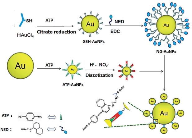
Fig. 1 The schematic of NO<sub>2</sub><sup>-</sup> detection by Au satellite-like aggregate colorimetry
