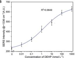
Fig. 7 (A) Response of the aptasensor to different concentrations of DEHP in 0.1 M pH 7.4 PBS. (B) Average of SERS peak intensity at  $\sim$ 1336 cm<sup>-1</sup> as a function of DEHP concentration. Error bar represents standard deviation (n=3).
