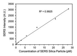
Fig. 5 Calibration curve of DEHP functionalized SERS silica particles in PBS. SERS intensity at 1336 cm<sup>-1</sup> with increasing concentration of the DEHP functionalized SERS silica particles. Error bar represents standard deviation (n = 3).
