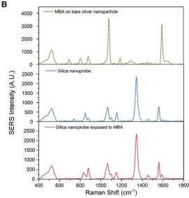
Fig. 6 Stability of the DEHP functionalized SERS silica particles. (A) SERS intensity at 1336 cm<sup>-1</sup> of the SERS silica particles after 1 h exposure to PBS (0.1 M, pH 7.4) with 0.1 M, 0.2 M, 0.5 M, and 0.7 M NaCl. (B) SERS spectra of Ag nanoparticles after 1 h exposure to 0.5 mM 4-MBA, and SERS silica particles after no exposure and exposure to 0.5 mM 4-MBA.
