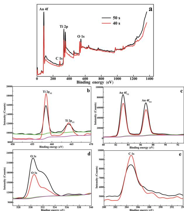
Fig. 4 (a) XPS survey spectra of the 40 s Au/TiO<sub>2</sub> NTs and the 50 s Au/TiO<sub>2</sub> NTs heterostructures and high-resolution spectra of (b) Ti 2p, (c) Au 4f, (d) O 1s, and (e) C 1s.
