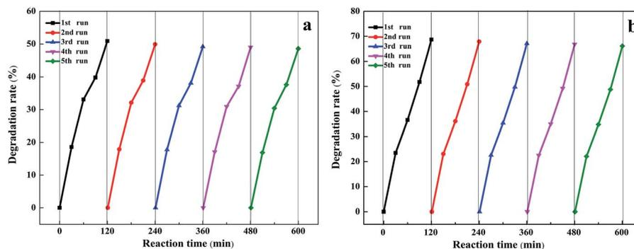
Fig. 7 Photostability and catalytic stability of (a) 40 s Au/TiO<sub>2</sub> NTs and (b) 50 s Au/TiO<sub>2</sub> NTs for photoelectrocatalytic degradation of nitrobenzene.
