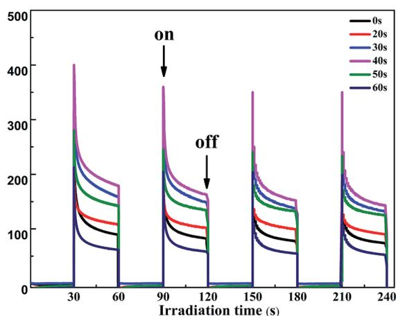
Fig. 3 Photocurrent response of the two-step TiO<sub>2</sub> NTs and the Au/TiO<sub>2</sub> NTs at an applied potential of 0.5 V under the irradiation of UV light and a Ag/AgCl electrode was used as a reference electrode.
