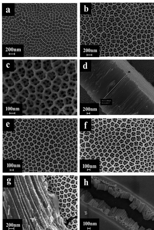
Fig. 1 SEM images of: (a) TiO<sub>2</sub> NTs; (b) 20 s Au/TiO<sub>2</sub> NTs; (c) 30 s Au/TiO<sub>2</sub> NTs; (d) side view of 30 s Au/TiO<sub>2</sub> NTs; (e) 40 s Au/TiO<sub>2</sub> NTs; (f) side view of 50 s Au/TiO<sub>2</sub> NTs; (g) 50 s Au/TiO<sub>2</sub> NTs; (h) 60 s Au/TiO<sub>2</sub> NTs.
