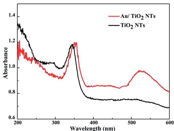
Fig. 5 UV-vis diffuse reflectance spectra of the  $\text{TiO}_2$  NTs and the Au/ $\text{TiO}_2$  NTs.
