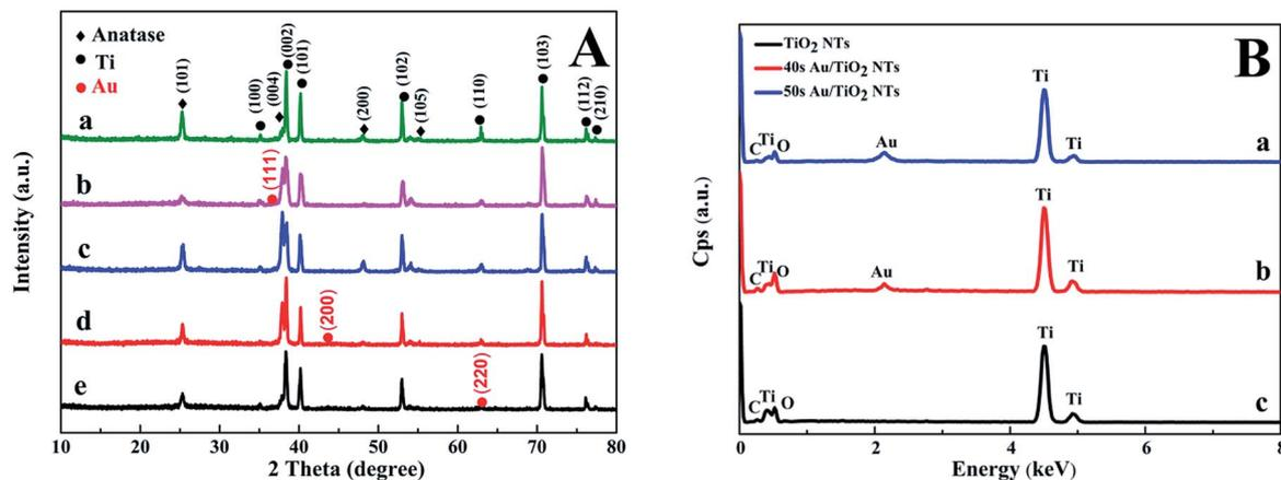
Fig. 2 (A) XRD patterns of: (a) 20 s Au/TiO<sub>2</sub> NTs; (b) 30 s Au/TiO<sub>2</sub> NTs; (c) 40 s Au/TiO<sub>2</sub> NTs; (d) 50 s Au/TiO<sub>2</sub> NTs; (e) 60 s Au/TiO<sub>2</sub> NTs. (B) EDS spectrum of: (a) TiO<sub>2</sub> NTs; (b) 40 s Au/TiO<sub>2</sub> NTs; (c) 50 s Au/TiO<sub>2</sub> NTs.
