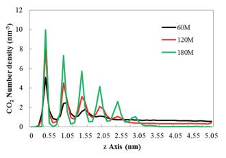
Fig. 3 The  $CO_2$  density profile along the z axis under no external electric field. "60M", "120M", "180M" represent system models containing 60, 120 and 180  $CO_2$  molecules in this paper, respectively.
