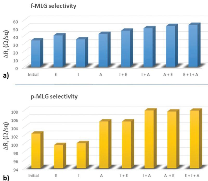
**Fig. 6** Selectivity analysis for cancer marker detection by monitoring the sheet resistance value for the three types of organics in various combinations with f-MLG (a) and p-MLG-based (b) electrodes: single solutions of ethanol (E), isopropanol (I), acetone (A); double solutions – E + I, E + A, and A + I; and the triple solution – E + I + A.
