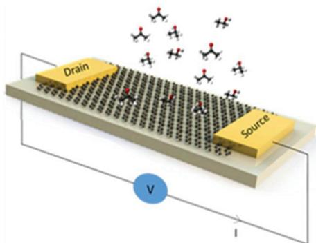
**Fig. 5** A schematic design of the flat or patterned MLG-based sensors for E/I/A-containing cancer marker detection. Graphene is placed on a flexible PVC substrate of  $25 \mu\text{m}$  thickness. A two-point measurement concept was used for the *in situ* electrical characterization of CM-induced graphene electrodes and its selectivity analysis.
