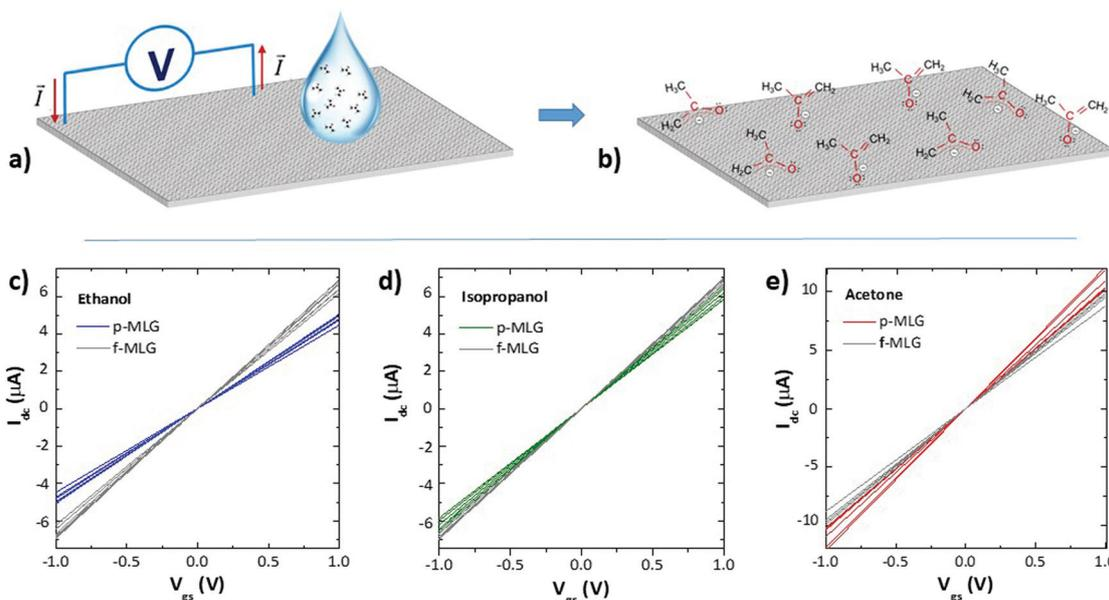
Fig. 3 The schematic representation of the two-point measurement concept (a) for the *in situ* electrical characterization of VOC-induced graphene electrodes (c, d); electron-induced reorientation of acetone while applying  $\pm 1$  V (b). The  $I_{dc}$  versus  $V_{gs}$  curves of the flat and patterned graphene electrodes influenced with exposure to  $1.4\text{--}3.3 \times 10^5$  ppm of VOC solutions: ethanol (c), isopropanol (d) and acetone (e).
