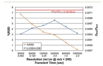
Fig. 5 Effect of increasing mass resolution setting (specified at m/z =200 Da) on the accuracy and precision of the <sup>235</sup>U/<sup>238</sup>U isotope ratio measurement. Each data point represents 3 acquisitions, each of which consisted of 10 scans of 10 microscans. CRM 129a test solution  $= 100 \text{ ng mL}^{-1}$ . Conditions: discharge current = 30 mA, solution flow rate = 30  $\mu$ L min<sup>-1</sup>, and sheath gas flow rate = 0.5 L min<sup>-1</sup>.
