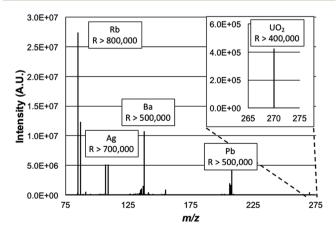
Fig. 2 Representative mass spectrum of a multi-element solution containing 500 ng mL $^{-1}$  each of Rb, Ag, Ba, Pb and U. The spectrum was taken in 'full scan' mode using a resolution setting of 500 000, specified for m/z=200 Da. Conditions: discharge current =30 mA, solution flow rate  $=30~\mu L~min^{-1}$ , and sheath gas flow rate  $=0.5~L~min^{-1}$ .
