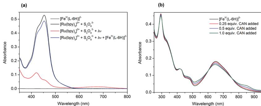
Fig. 2 (a) UV-vis spectra demonstrating the photochemical oxidation of [Ru(bpy)<sub>3</sub>]<sup>2+</sup> (0.05 mM) to [Ru(bpy)<sub>3</sub>]<sup>3+</sup> by persulfate (0.2 mM) with the following reduction by the catalyst (0.5 μM). The spectrum of the catalyst (0.5 μM) is given for comparison in grey. (b) UV-vis spectra demonstrating titration of the catalyst [Fe<sup>IV</sup>(L-6H)]<sup>2-</sup> (0.02 mM) by CAN.
