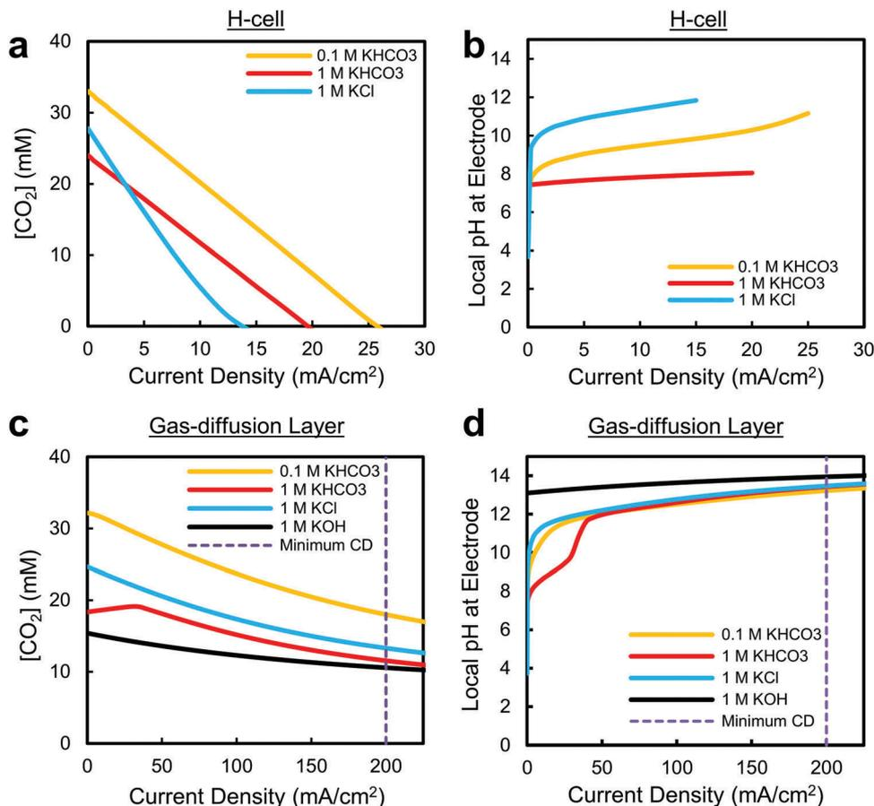
Fig. 3 Simplified predictions of the electrode concentration of  $\text{CO}_2$  and pH for commonly-used electrolytes as a function of current density in an (a and b) H-cell with a  $50 \mu\text{m}$   $\text{CO}_2$  diffusion thickness and, (c and d) a gas-diffusion layer with a  $50 \text{ nm}$   $\text{CO}_2$  diffusion thickness and liquid diffusion layer of  $200 \mu\text{m}$ . A Faradaic efficiency of  $\text{CO}_2$ -to- $\text{CO}$  of 90% is assumed.
