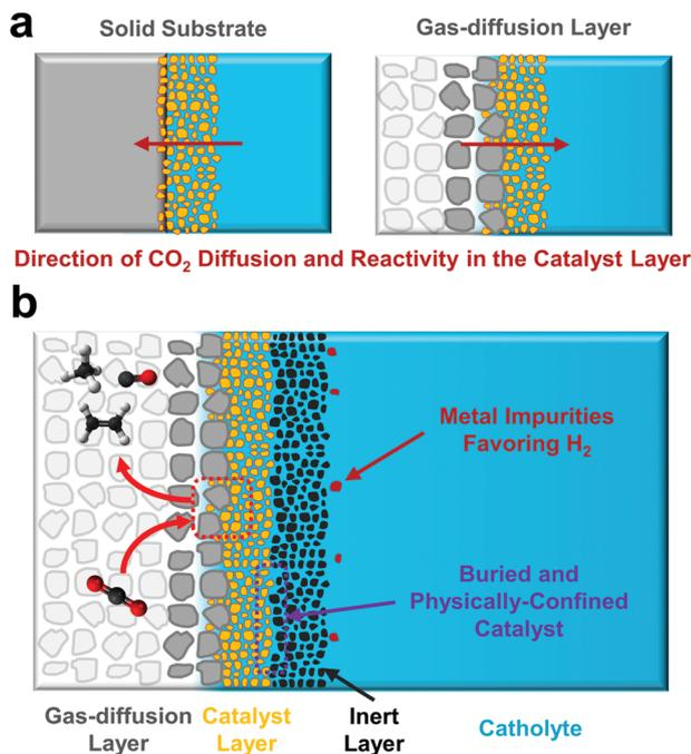
Fig. 5 (a) Schematic of the directional change in  $\text{CO}_2$  transport for fully-aqueous and gas-diffusion layer  $\text{CO}_2$  reduction catalysts. (b) Potential advantages of a change in the  $\text{CO}_2$  transport and reaction direction inside a catalyst layer. A buried catalyst layer may be inherently more stable and protected from both contaminants and restructuring while still having access to  $\text{CO}_2$ .
