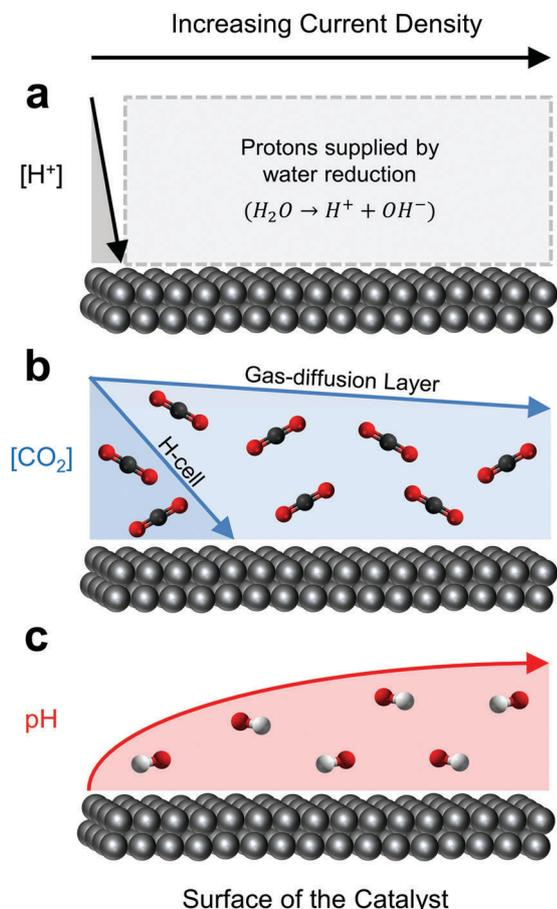
Fig. 1 The relative effect of current density on the reaction (a) proton source, (b) concentration of CO<sub>2</sub> and (c) pH at the surface of a CO<sub>2</sub> reduction catalyst.
