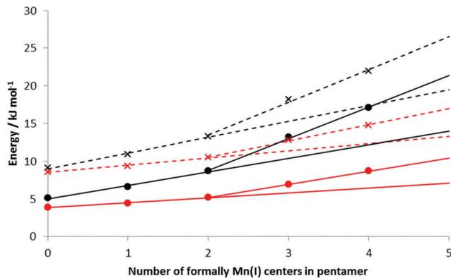
Fig. 7 Hydrogen binding energies and enthalpies for loadings of 1 H<sub>2</sub> per Mn and 2 H<sub>2</sub> per Mn on our pentameric BSMs. Black: 5 H<sub>2</sub>, red: 10 H<sub>2</sub>, crosses: HBE, circles: enthalpies. Dashed lines show extrapolation of the different trends in the HBE to 100% Mn(I) concentration. Solid lines show extrapolation of the different trends in the enthalpies to 100% Mn(I) concentration.
