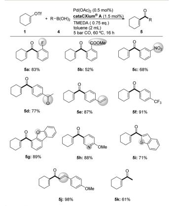
Scheme 3 Pd-catalyzed synthesis of 1-cyclohexenyl aryl ketones. Reaction conditions: 0.5 mmol 1, 1.2 eq. of 4, in argon. Isolated yields.
