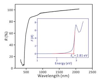
Fig. 3 UV-vis-NIR transmittance spectrum of  $Cs_3VO(O_2)_2CO_3$ . The inset shows an optical diffuse reflectance spectrum of  $Cs_3VO(O_2)_2CO_3$ .
