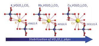
Fig. 2 Ball-and-stick models revealing the effect of the size of alkali metal cations on the stability of VO $_3$ (O $_2$ ) $_2$  pbps in A $_3$ VO(O $_2$ ) $_2$ CO $_3$ . While the shorter O–O distances in peroxo ligands due to the smaller coordination environment of K $^+$  result in more strained VO $_3$ (O $_2$ ) $_2$  pbps, the longer O–O distances in peroxo ligands attributed to the large Cs $^+$  generate less strained stable VO $_3$ (O $_2$ ) $_2$  pbps.
