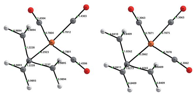
Fig. 8 Equilibrium geometries for  $(\eta^4-C_4H_6)$ Fe(CO)<sub>3</sub> at the B3LYP/6-311++G(2d,2p) level of theory, displaying delocalization indices at the usual levels of theory. The left structure corresponds to HF values, and the right to CCSD values. The Fe-C<sub> $\beta$ </sub> values are not displayed, and are commented in text.
