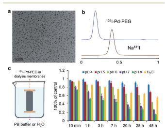
Fig. 1 (a) Representative TEM image of Pd nanosheets. (b) TLC images of free  $^{131}$ I and  $^{131}$ I labeled Pd nanosheets. (c) Stability test of  $^{131}$ I-Pd-PEG in PB buffer with different pH values through dialysis.
