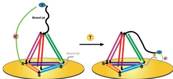
**Scheme 1** The E-nanoDNA sensor contains an electrode-bound, redox-reporter modified tetrahedral DNA nanostructure, with two functional strands (black and grey), that undergoes a target binding-induced conformational change on the electrode surface. This conformational change pulls the reporter (methylene blue, MB) close to the electrode surface (yellow disk), thereby producing a target-dependent change in current when the sensor is interrogated by square wave voltammetry.
