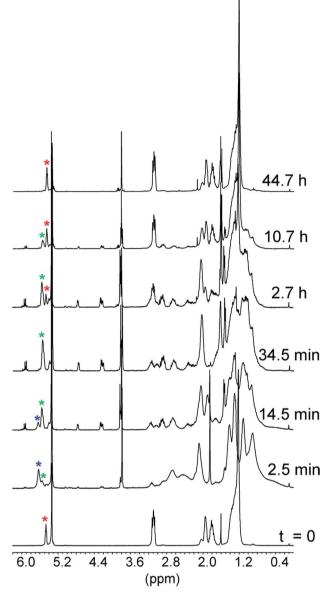
Fig. 2  $^{1}$ H NMR monitoring of the reaction of 5 mM 1 with 5 mM 2 (X = OCH<sub>3</sub>) in CD<sub>2</sub>Cl<sub>2</sub> at 25 °C. The trace at time zero is the spectrum of catenand 1. The asterisks denote the signals of the double bond protons: red = catenand 1, blue = B' and green = B''.
