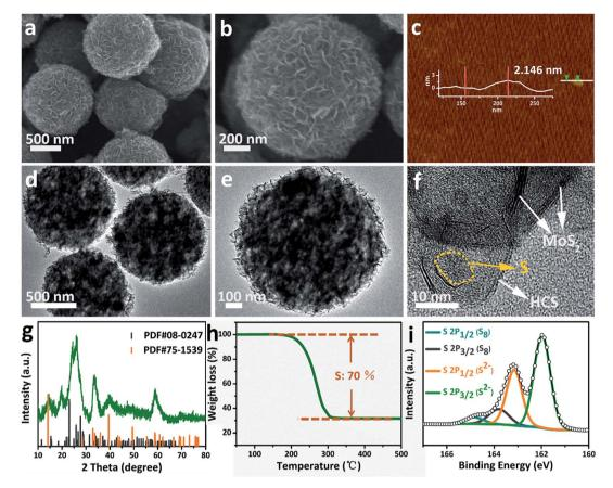
Fig. 2 (a and b) FESEM, (d-f) TEM images, (g) XRD, (h) TGA and (i) XPS spectra of the S/MoS<sub>2</sub>@HCS composite. (c) AFM image of the MoS<sub>2</sub>@HCS composite after a sonication treatment.
