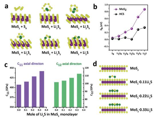
Fig. 4 (a) Schematics of various polysulfide conformations on  $MoS_2$ . (b) Binding energies for  $Li_xS_n$  species at six different lithiation stages  $(S_8, Li_2S_6, Li_2S_6,$
