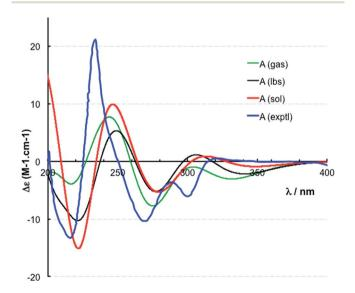
Fig. 4 Experimental (exptl, blue) and computed ECD spectra of (10S,11S,23S)-caulamidine A at the B3LYP/6-31G\*\* (gas, green) and B3LYP/6-311++G\*\* (lbs, black) levels in the gas phase and at the B3LYP-SCRF(COSMO)/6-311++G\*\*/B3LYP/6-311++G\*\* (sol, red) level in MeOH.
