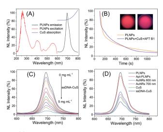
Fig. 2 (A) Excitation and emission spectra of PLNPs and absorption spectra of CuS nanoparticles. (B) Afterglow property of PLNPs and PLNPs-CuS nanoprobes in the presence of AFT B1. (C) The luminescence quenching of CuS NPs to PLNPs. (D) Comparison of the quenching effect of AuNRs and CuS NPs on the luminescence of PLNPs.
