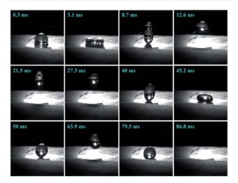
Fig. 4 Bounce dynamics of a water droplet impacting with the PF coupled with sprayed SiO<sub>2</sub> coatings and the MPA surface.
