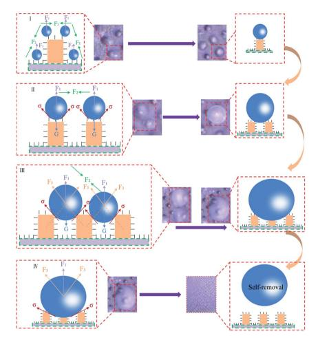
Fig. 8 The antifogging behaviors of the PF coupled with sprayed  $SiO_2$  coating and the MPA. Here,  $F_1$  is the repulsion force of the material itself,  $F_2$  is the intermolecular attraction,  $F_3$  is the repulsion force of the micro-pillared arrays,  $\sigma$  is surface tension and G is gravity.
