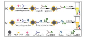
Fig. 1 Schematic illustrations of IMB (1) and BSA-IMB (2) for detecting AFB $_1$ .
