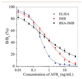
Fig. 2 Immunoassay calibration curves for AFB<sub>1</sub>.
