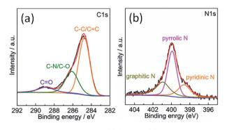
Fig. 4  $\,$  XPS core level spectra of (a) C 1s and (b) N 1s of the surface of as-obtained porous carbon sample.
