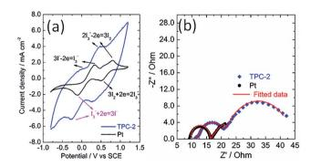
Fig. 5 (a) Cyclic voltammograms for TPC and Pt electrode at a scan rate of 100 mV s<sup>-1</sup> in acetonitrile solution containing 10 mM LiI, 1 mM  $I_2$ , and 0.1 M LiClO<sub>4</sub> with a platinum wire and a SCE electrode used as counter electrode and reference electrode, respectively; (b) Nyquist plots for electrochemical impedance spectra of the symmetrical cells with two identical TPC-2 and Pt electrodes.
