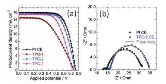
Fig. 6 (a) Characteristic photocurrent density–voltage curves of the DSCs with TPC CEs of different thicknesses and Pt CE, measured under solar simulator illumination of 100 mW cm<sup>-2</sup> (AM 1.5G); (b) electrochemical impedance spectra of DSCs using TPC-2 and Pt CEs measured under light irradiation, at open-circuit voltage; dots present experimental results, and solid lines show fitted results.
