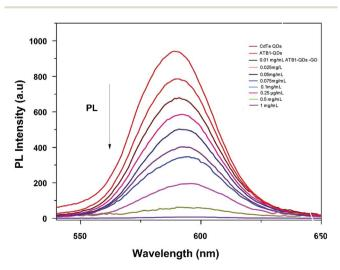
Fig. 5 Characterization of graphene oxide–quantum dots: monitoring the fluorescence quenching of quantum dots at various graphene oxide (0.01–1 mg ml<sup>-1</sup>) concentrations using PL spectroscopy.
