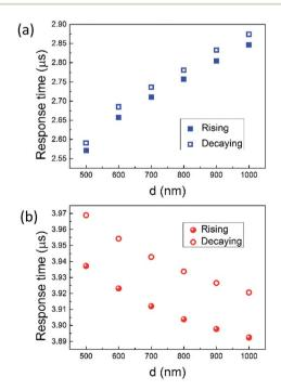
Fig. 10 Rising and decaying time as function of  $\emph{d}$  in the structure without air trench (a) and with air trench (b).
