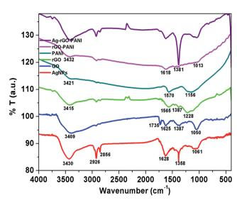
Fig. 2 FTIR spectra showing the various functional groups present in AgNPs, GO, rGO, PANI and their involvement in the preparation of rGO-PANI, and AgNPs-rGO-PANI nanocomposite.
