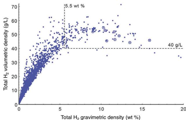
Fig. 2 Theoretical total volumetric vs. gravimetric capacities for various materials at 77 K and 35 bar, compared with the DOE 2025 system targets (5.5 wt% and  $40 \text{ g L}^{-1}$ , as outlined by dashed lines). Adapted with permission from J. Goldsmith, A. G. Wong-Foy, M. J. Cafarella and D. J. Siegel, *Chem. Mater.*, 2013, **25**, 3373. Copyright 2008 American Chemical Society.
